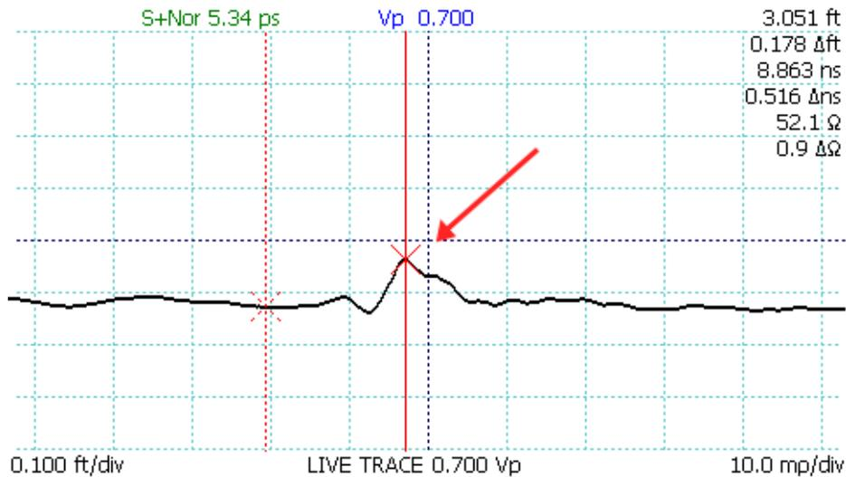
**Figure 7.4.** Normal SMA female barrel interconnect measuring 52.1 ohms.
